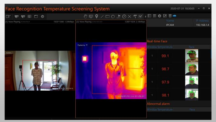
The interface shows both thermal and visual images of the individual being scanned. It can also display multiple temperature readings for the individual with real-time facial images.
